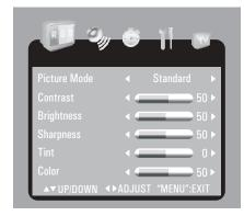
Picture Mode: Select from preset screen display settings to match the type of show you are watching
